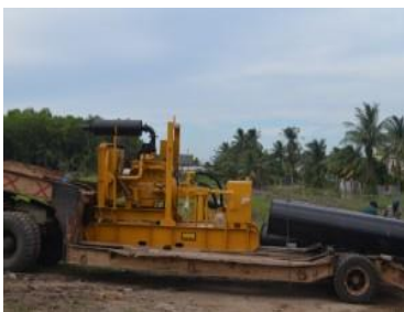
Hydra Flow Mobile pump used in Guyana
