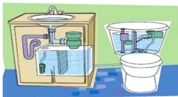
Fig. 11. The Aquas™ toilet uses gray water from the sink for toilet flushing
